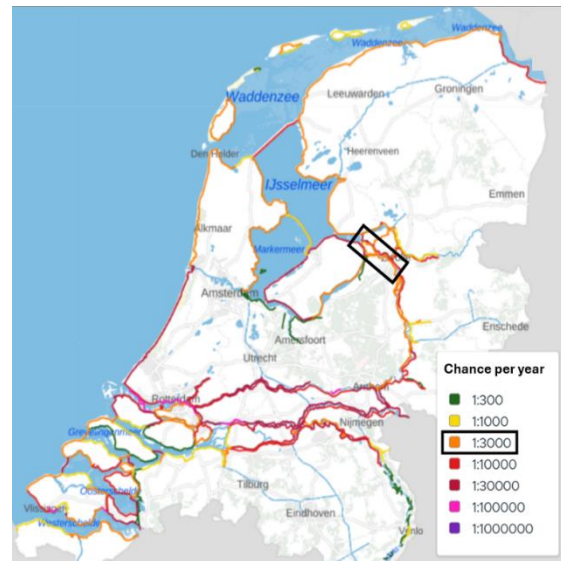
Figure 7. Map of minimal water safety standards for primary dikes. The project location Mastenbroek-IJssel is displayed in black. (Normering, n.d.)
