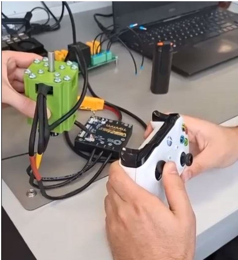
X-box controller implementation for motor control, by Emiel Visser.
