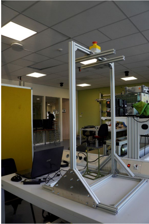
Aluminum profile frame, designed and manufactured by Roman Kim and Ky Do.
