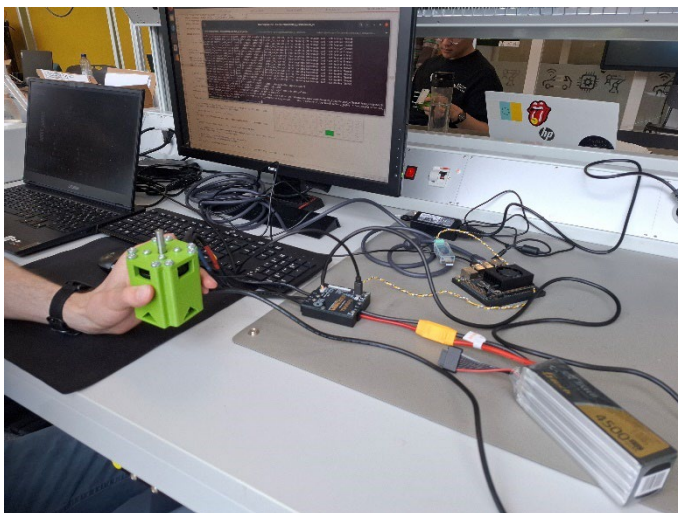
Emiel Visser, testing motor control with Jetson Nano, a powerful computer often used in robotics projects.
