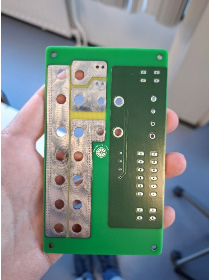
Empty printed circuit board (PCB), designed and manufactured by Tim Roordink.
